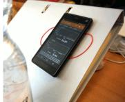
Figure 2.12: (top) As long as  $\theta$  is smaller than the angle of friction the blue block does not slide. (bottom) Placing my cell phone on two rubber bands on a folder provides a maximum angle of about 33°, i.e.  $\mu \simeq 0.5$ . Using PhyPhox and a cell phone one can easily measure  $\theta_c$  and  $\mu$  for other combinations of materials.
