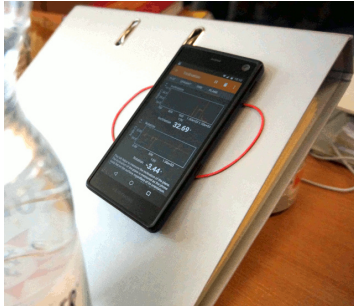
Figure 2.12: (top) As long as \theta is smaller than the angle of friction the blue block does not slide. (bottom) Placing my cell phone on two rubber bands on a folder provides a maximum angle of about 33^\circ , i. e. \mu \simeq 0.5 . Using PhyPhox and a cell phone one can easily measure \theta_c and \mu for other combinations of materials.
