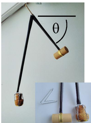
Figure 6.9: Setup of the kitchen pendulum.
