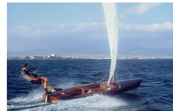
Gwicke commonswiki, public domain Figure 2.22: A sailor stacking out in a trapeze in order to minimize the heeling of his sailboat.
