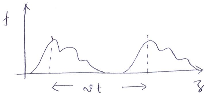
$f(z, t)$  represents the wave which has a propagation direction  $z$  and velocity  $v$ . This travelling wave can be mathematically represented as:
