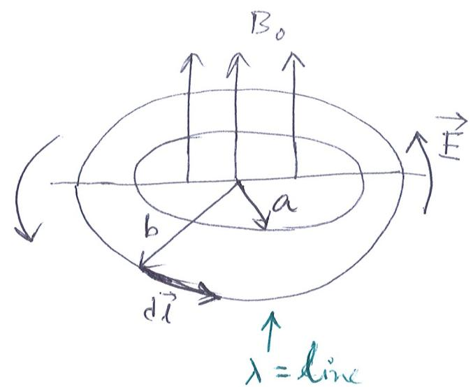
→ When we turn off the magnetic field, the magnetic flux will change through the loop. And this induces an electric field in it. As this ~~is disk contains~~ wheel contains some charge, for which  $\lambda$  is the line charge density, it will feel some force. And this force will induce the torque and the wheel will rotate.
