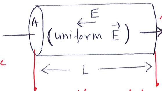
this can be thought as a schematic of a conducting wire.
