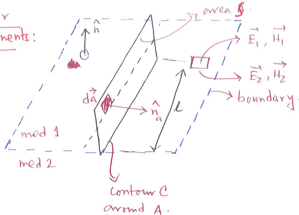
A very thin Amperean loop is considered. Then for the electric field we get :
