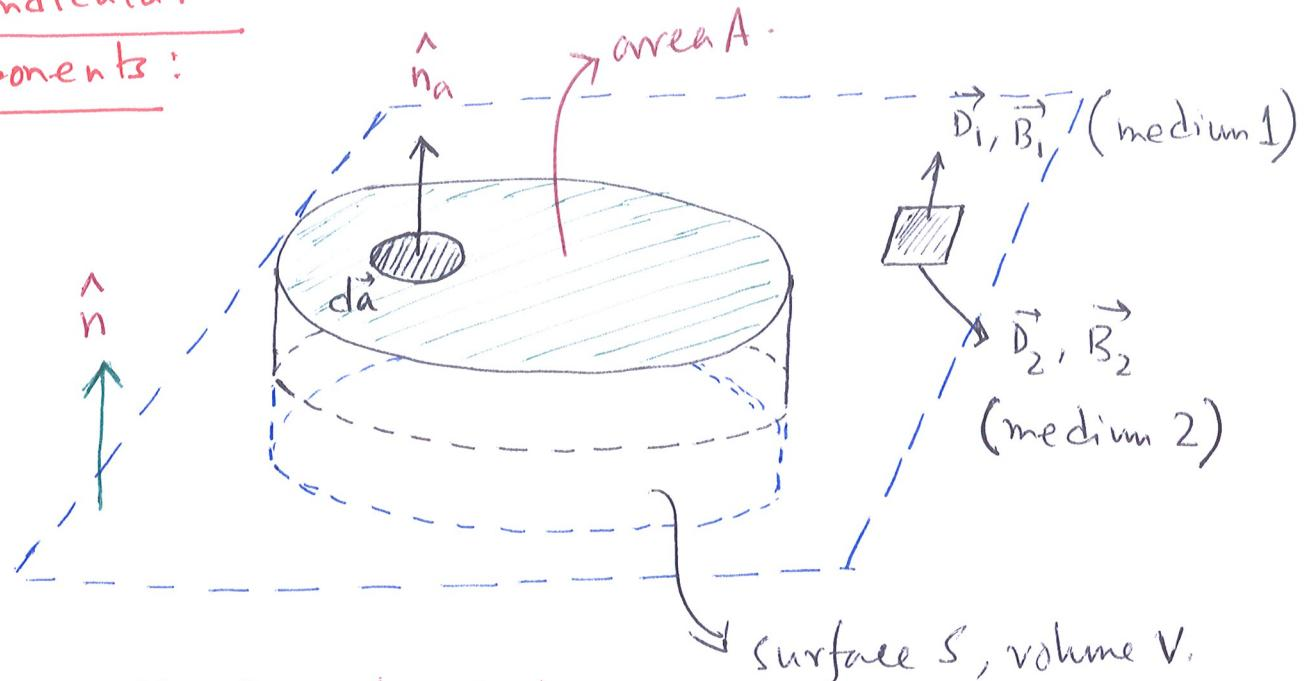
Schematic to represent boundary at two mediums. And to look at the ~~discontinuity~~ ~~xxx~~ normal components of the fields.
