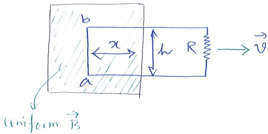
In this case a resistor  $R$  is pulled with a speed  $\vec{v}$  to the right through an uniform magnetic field  $\vec{B}$  which points into the page.
