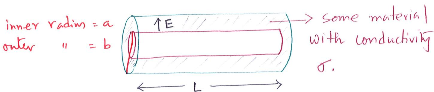
(two concentric cylinders are maintained at a potential difference  $V$ )
