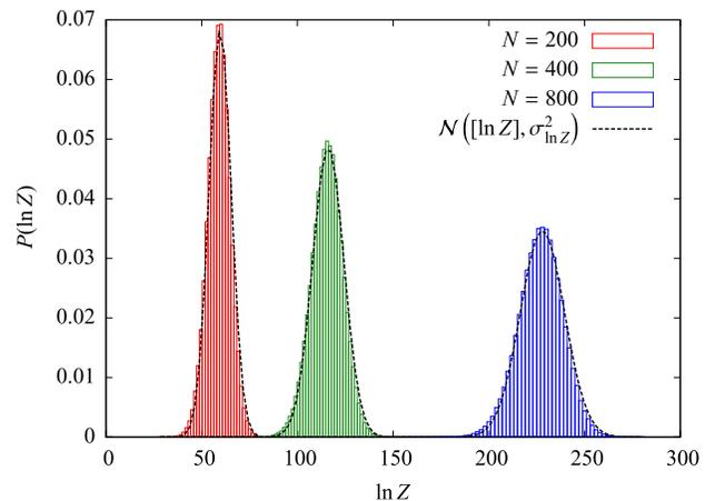
FIG. 4 (color online). Measured probability densities of the entropy  $\ln Z$  for various lengths. The dashed lines are normal distributions with the same mean values and variances (no fit involved).
