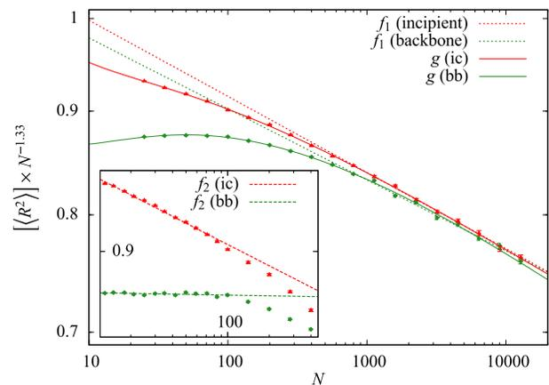
FIG. 3 (color online). Mean squared end-to-end distance vs number of steps for SAWs on incipient critical clusters (red) and backbones (green) on a log-log scale. The lines show the results from different least-squares fits.  $f_1$ : Eq. (2) with  $N = 800$ – $12\,800$  (ic) and  $N = 1131$ – $12\,800$  (bb);  $f_2$  (inset): Eq. (2),  $N = 13$ – $100$ ;  $g$ : Eq. (3),  $N = 25$ – $12\,800$ . The factor  $N^{-1.33}$  ( $\approx N^{-2\nu}$ ) serves to magnify the differences.
