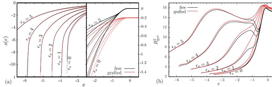
Figure 4. (a) Microcanonical entropy  $s(e) = \ln g(e)/N$ . Since  $g(e)$  spans many orders of magnitude at low energies, the ordinate is divided into two different regimes. (b) Squared radius of gyration  $R_{\text{gyr}}^2(e)$  versus energy.
