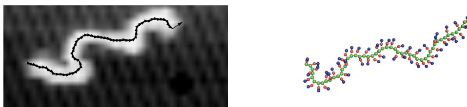
**Figure 1.** Scanning tunneling microscopy image of a P3HT 50-mer on Au(001) (left) and elongated 50-mer conformation on a surface obtained by Monte Carlo simulations (right).
