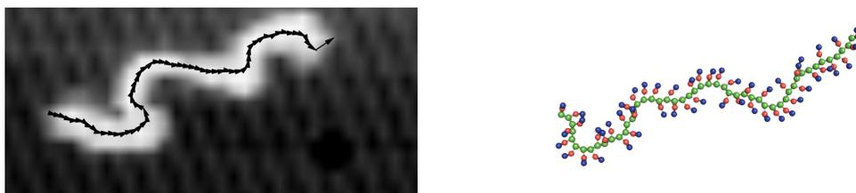
**Figure 1.** Scanning tunneling microscopy image of a P3HT 50-mer on Au(001) (left) and elongated 50-mer conformation on a surface obtained by Monte Carlo simulations (right).
