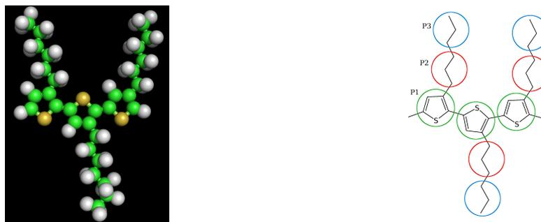
**Figure 3.** Atomistic structure of a P3HT 3-mer in bead-stick representation (left) and a sketch of the three beads per monomer coarse-grained Model B (right).
