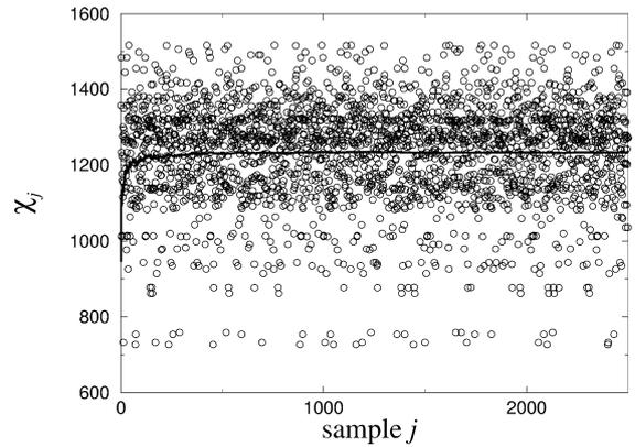
Fig. 3. Distribution of the susceptibility for the different disorder realizations of the Ising model with  $L = 96$  and a concentration of magnetic bonds  $p = 0.7$ . The average value over the samples  $\bar{\chi}$  is shown by the black line.
