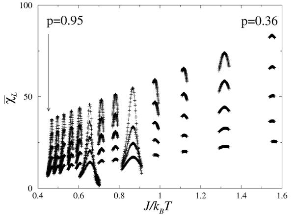
Fig. 1. Variation of the average magnetic susceptibility  $\bar{\chi}_L$  versus the coupling strength  $K = J/k_B T$  for several concentrations  $p$  and  $L = 8, 10, 12, 14, 16, 18, 20$ . For each value of  $p$  and each size, only one value of  $K$  has been simulated: the extension of the  $K$  values has been obtained by the standard histogram reweighting technique.
