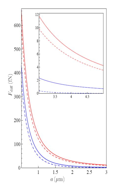
Predicted values of the differential Casimir force for the configuration with structured Au-Si plate
