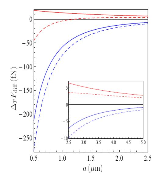
Thermal corrections to the differential Casimir force computed at room temperature using the plasma model for Au with disregarded and taken into account free charge carriers in dielectric Si (top pair of solid and dashed lines, respectively) and using the Drude model for Au with disregarded and included free charges in dielectric Si (bottom pair of solid and dashed lines, respectively) are shown as functions of separation. The Si overlayer is 100nm thick.
