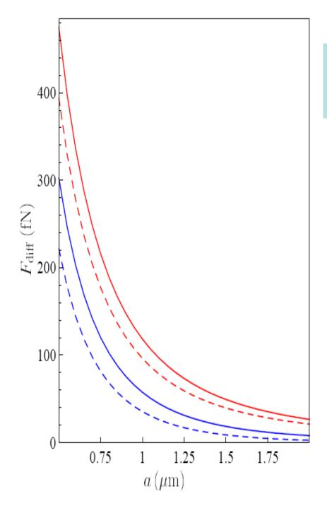
Predicted values of the differential Casimir force for the configuration with additional silica layer
