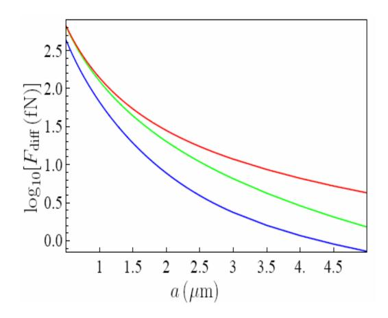
Logarithms of the differential Casimir forces computed at 300K using the plasma and Drude models for Au with disregarded free charges in dielectric Si are shown as functions of separation by the top and bottom lines, respectively. The medium line shows common computational results for the differential Casimir force at zero temperature. The Si overlayer is 100nm thick.
