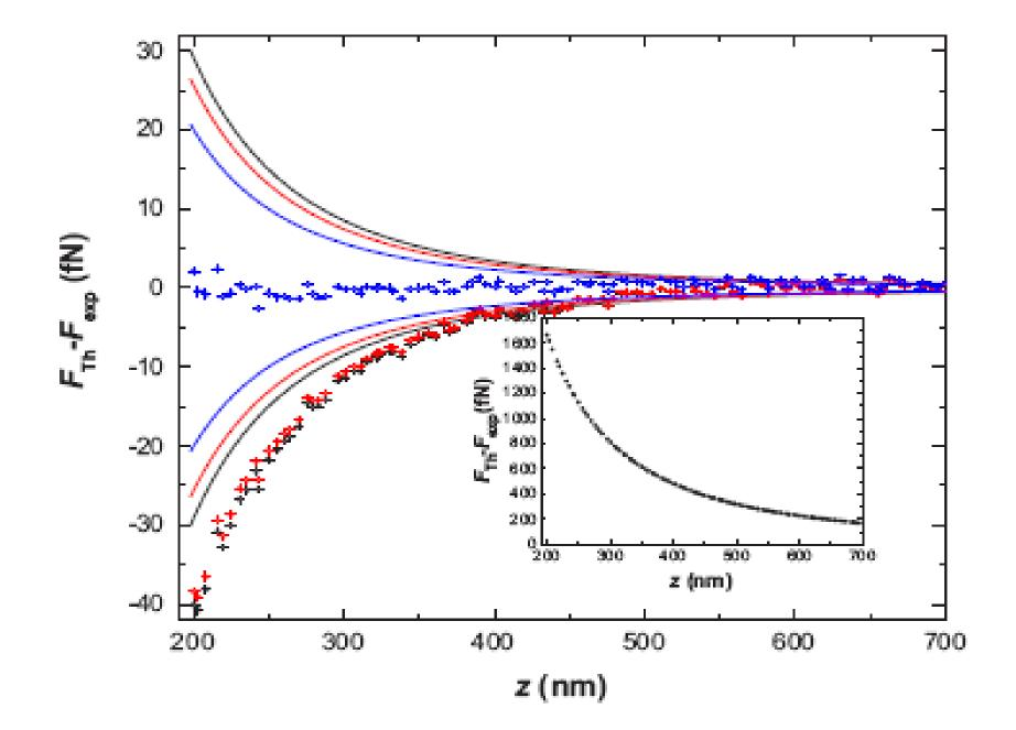
3. Proposed differential force measurement between Au sphere and structured plate with a Si overlayer
