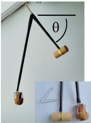
Figure 6.19: Setup of the kitchen pendulum.
