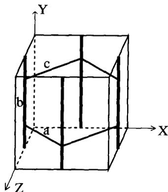
Fig. 1. Schematic view of the channel system within one unit cell of silicalite.
