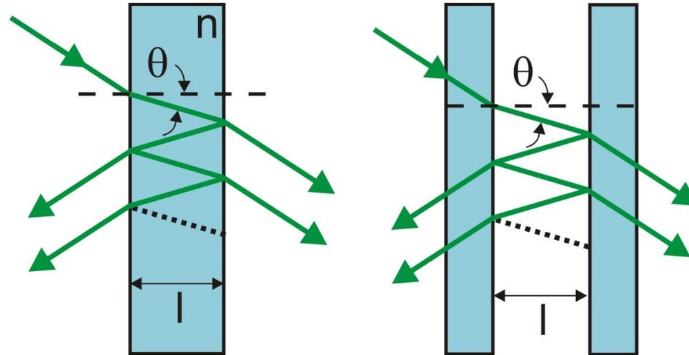
The functionality of a Fabry-Pérot interferometer is based on multi-beam interference on two plane-parallel surfaces.
