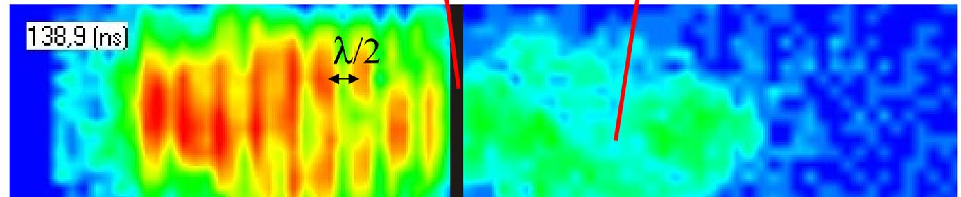
**standing spin wave:** wave is reflected back and forms a standing wave
