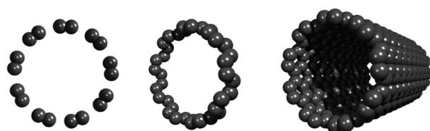
**Figure 1.** Structure of the CNT (9,9) carbon nanotube. Left: Flat single ring formed by 18 carbon atoms. Middle: Double ring formed by two flat single rings. Right: Carbon nanotube consisting of 10 double rings.
