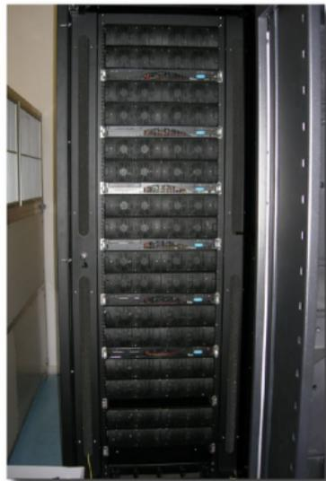
JANUS, a modular massively parallel and reconfigurable FPGA-based computing system.
