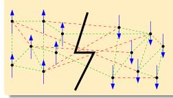
Then, a ground state is given by a configuration with minimal cut  $W^{\pm}$ , which divides the spins between the "up" and "down" states.
