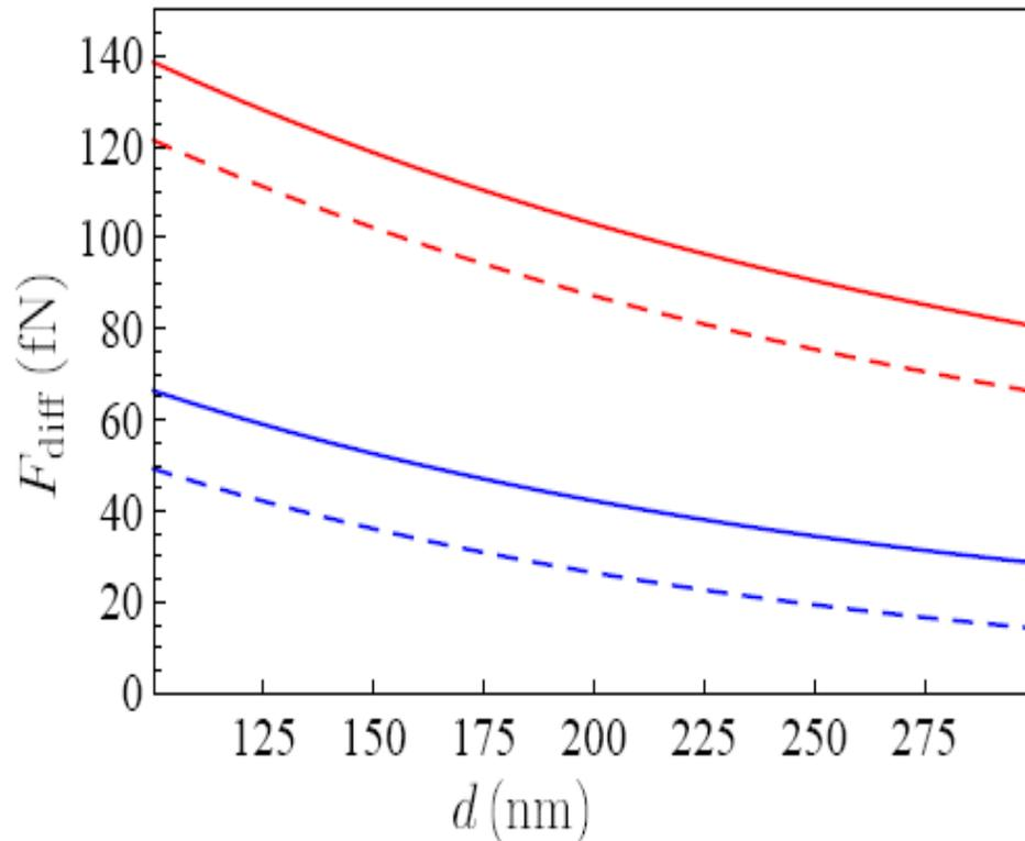
**Differential Casimir force computed at room temperature using the plasma model for Au with disregarded and taken into account free charge carriers in dielectric materials (top pair of solid and dashed lines, respectively) and using the Drude model for Au with disregarded and included free charges in dielectrics (bottom pair of solid and dashed lines, respectively) are shown as functions of overlayer thickness at the separation of one micrometer.**
