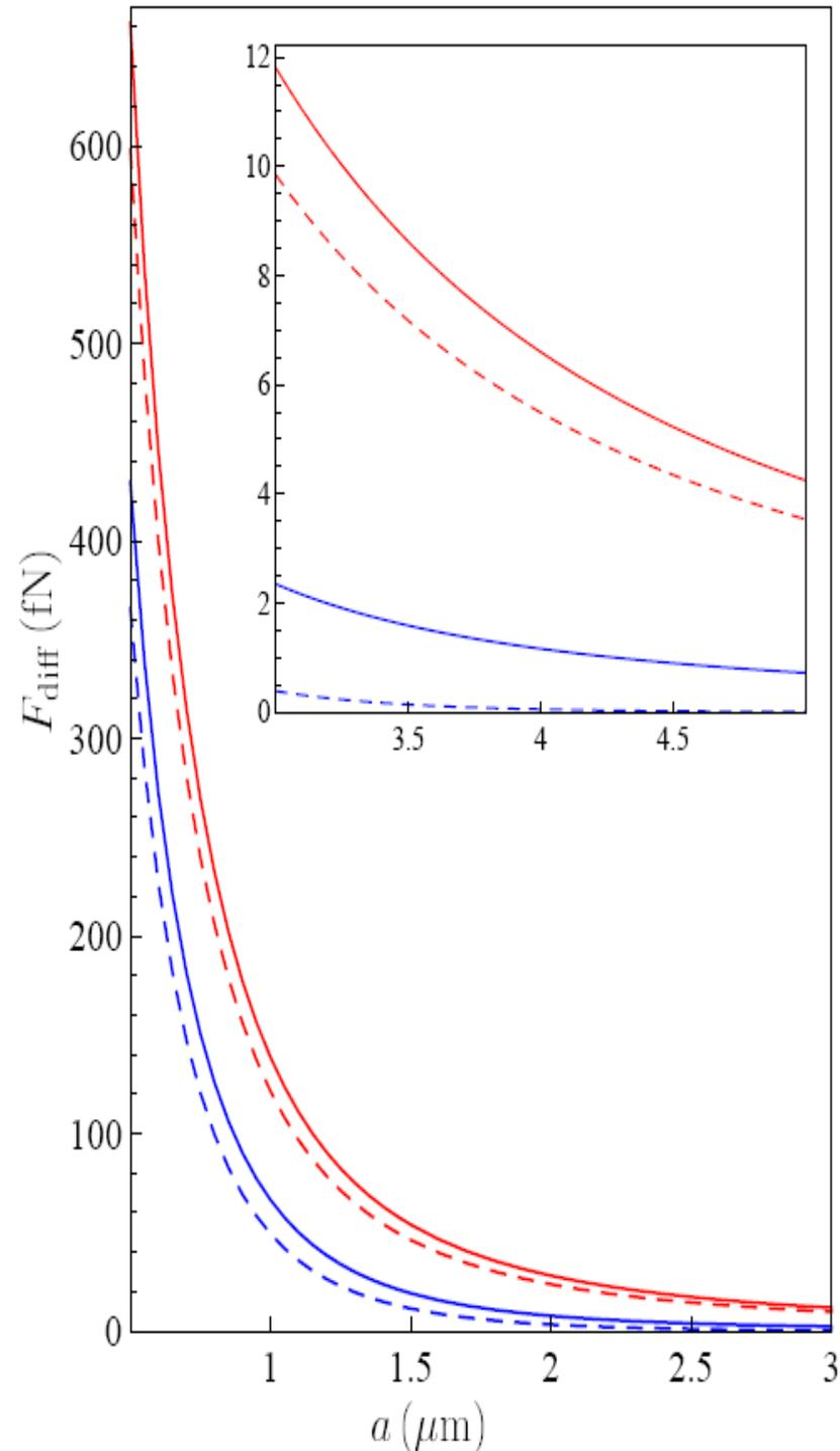
**Predicted values of the differential Casimir force for the configuration with structured Au-Si plate**
