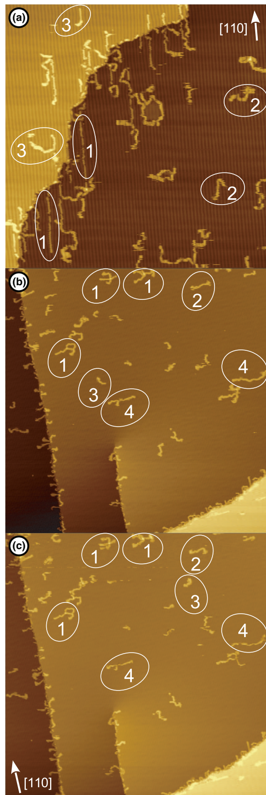
FIG. 5. STM images of in situ deposited P3HT molecules on the Au(001) surface. The images (b) and (c) are taken 15 min apart. For explanation see text. (a) 110 \times 110 \text{ nm}^2 , 50 pA, -1.5 \text{ V} . (b) and (c) 230 \times 230 \text{ nm}^2 , 50 pA, -2.0 \text{ V} .
