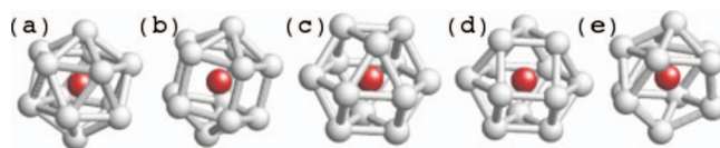
FIG. 2. Possible shell conformations ( r_c = 2.5\sigma ) of a monomer possessing 12 [(a)–(d)] or 11 (e) neighbors: (a) icosahedron, (b) elongated pentagonal pyramid (Ref. 28), (c) cuboctahedron (fcc), (d) triangular orthobicupola (Ref. 28) (hcp), and (e) incomplete icosahedron. Sticks illustrate shell contacts, not bonds.
